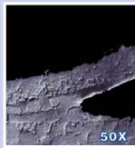
Shown here at 25X and 50X magnification, a strong and ductile single phase microstructure is formed in 316L stainless steel joints of an industrial heat exchanger brazed with Metglas MBF-51 amorphous brazing foil.
