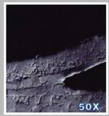
Shown here at 25X and 50X magnification, a strong and ductile single phase microstructure is formed in 316L stainless steel joints of an industrial heat exchanger brazed with Metglas MBF-51 amorphous brazing foil.
