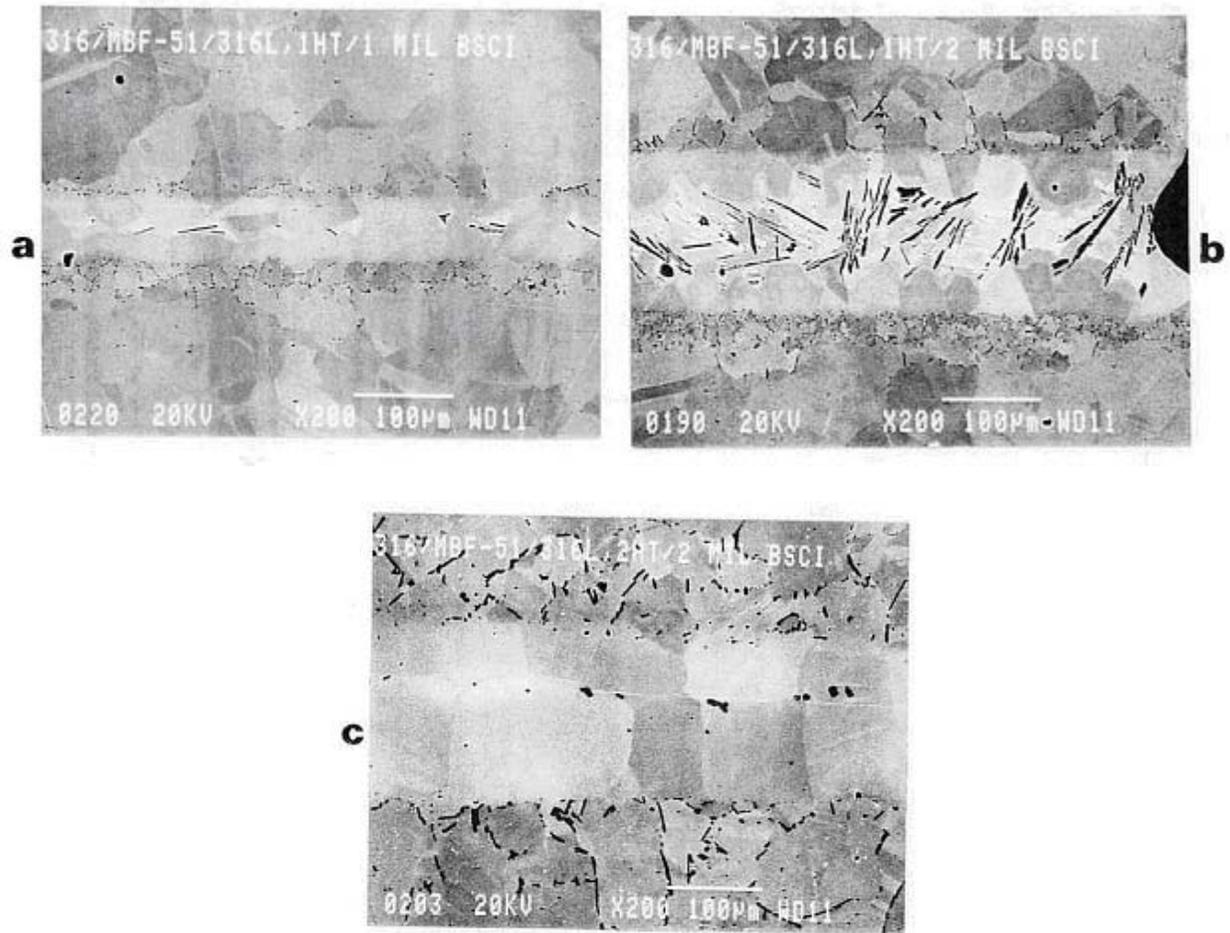
14. SEM micrograph of 316/MBSF-51/316 joints brazed using 25 (a) and 50  $\mu\text{m}$  (b) thick MBF-51 ribbon and a short brazing cycle; 50  $\mu\text{m}$  foil and a long brazing/annealing cycle were used in joint shown in (c). Note that a strong ductile single phase braze was formed when there was a small amount of boron in the joint and/or a long brazing time is used.<sup>17</sup>
