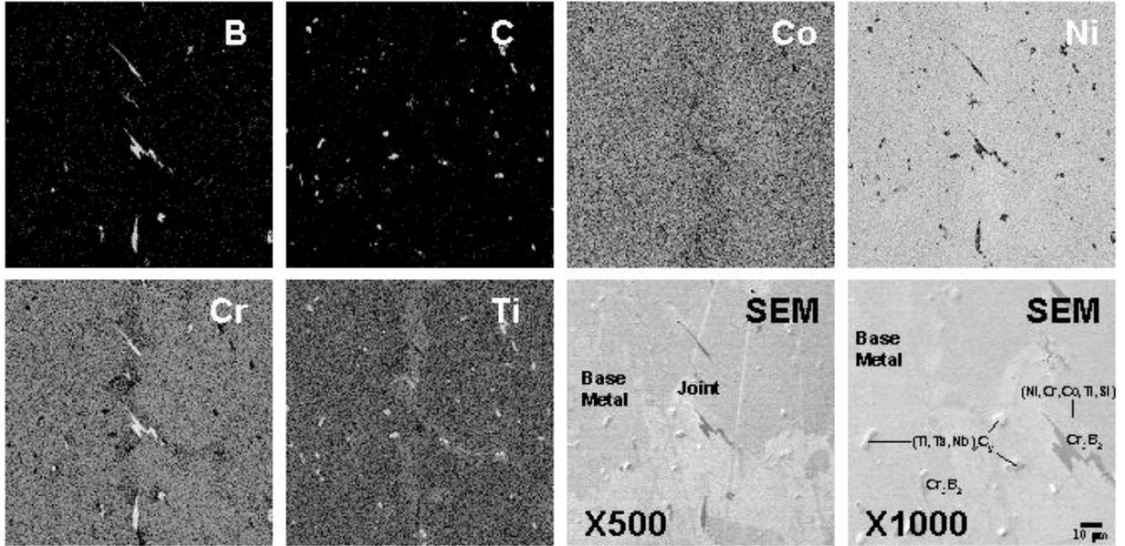
20. Microstructure of and elemental distribution in IN939/MBF-53/IN939 joints brazed at 1170°C for 15 min and annealed at 1070°C for 6 hours.
