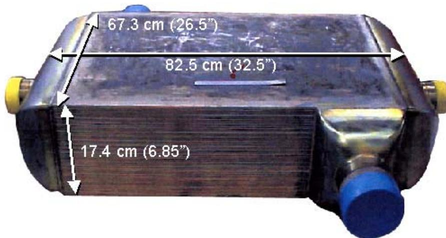
25. Two large heat exchangers brazed using side-by-side preplaced MBF-51 200 mm wide preforms.
