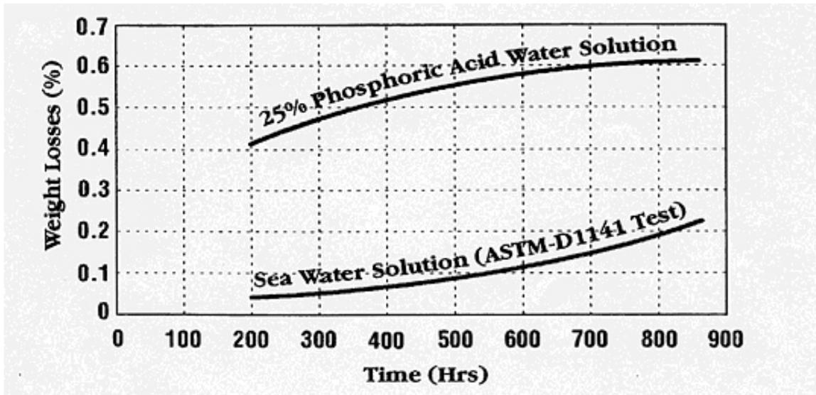
21. Weight losses of 316/MBF-51/316 Joints in a 25% water solution of phosphoric acid and sea water<sup>17</sup>.
