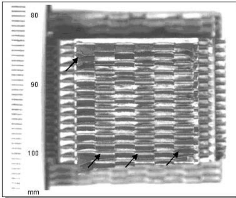
12. Samples of 436 stainless steel plate/fin samples after tensile testing: (a) 25- $\mu\text{m}$  thick MBF-20 foil. Unbraided area is seen (white arrow). Note that failure occurred in the lean fillets (black arrows). (b) 50 $\mu\text{m}$  MBF-20 foil: Failure occurred in the middle of the fin base metal (arrows) due to a large cross-section formed using sufficiently thick brazing foil.
