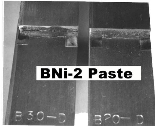
5. Fillets formed by MBF-20 foil and BNi-2 paste on 409 stainless steel joints brazed under -40°C FP 50:50 N<sub>2</sub>: H<sub>2</sub> atmosphere at 1115°C for 10 min. Note incomplete flow and crevices formed on a sample brazed with the paste.
