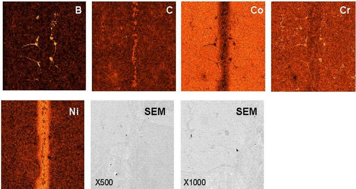
18. Microstructure of and elemental distribution in a X45/MBF-53/X45 joint brazed at 1170°C for 15 min and annealed at 1070°C for 6 hours.
