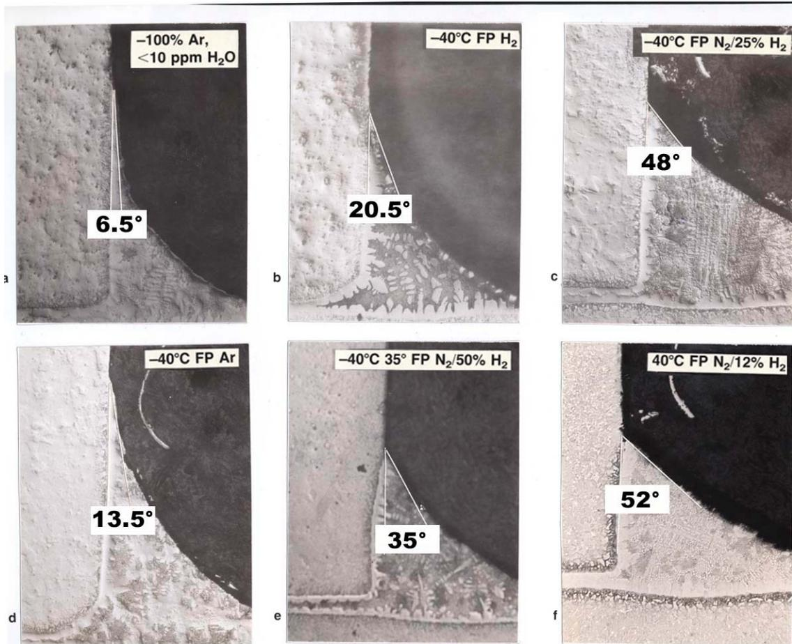
4. Contact angles formed by MBF-20 alloy on the vertical part of the T-type 409 stainless steel joints brazed under various atmospheres at 1115°C for 10 min. (100X).<sup>20</sup>
