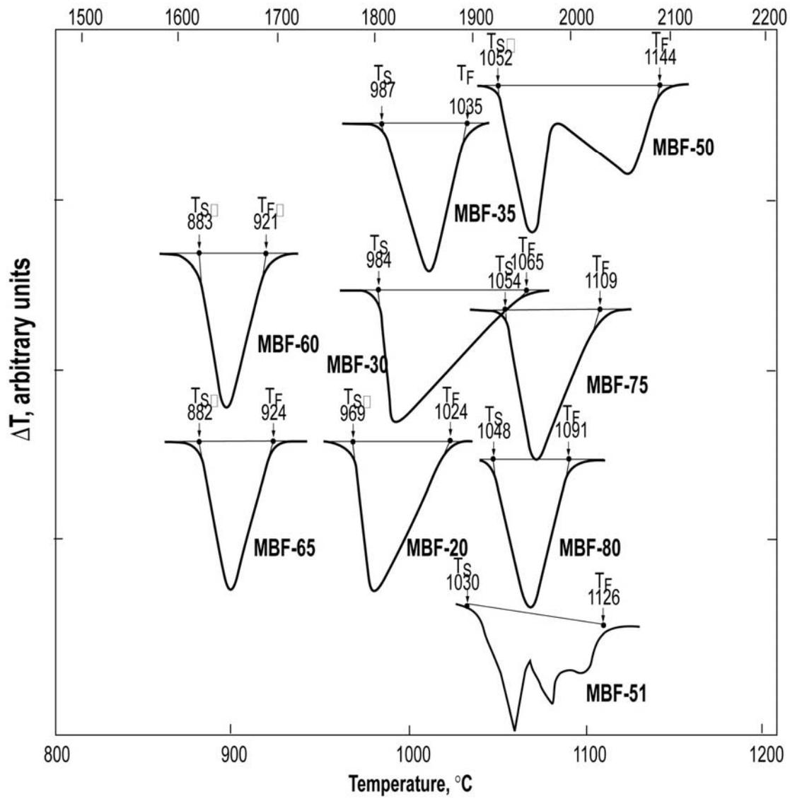
2. DTA melting troughs of some MBF alloys.
