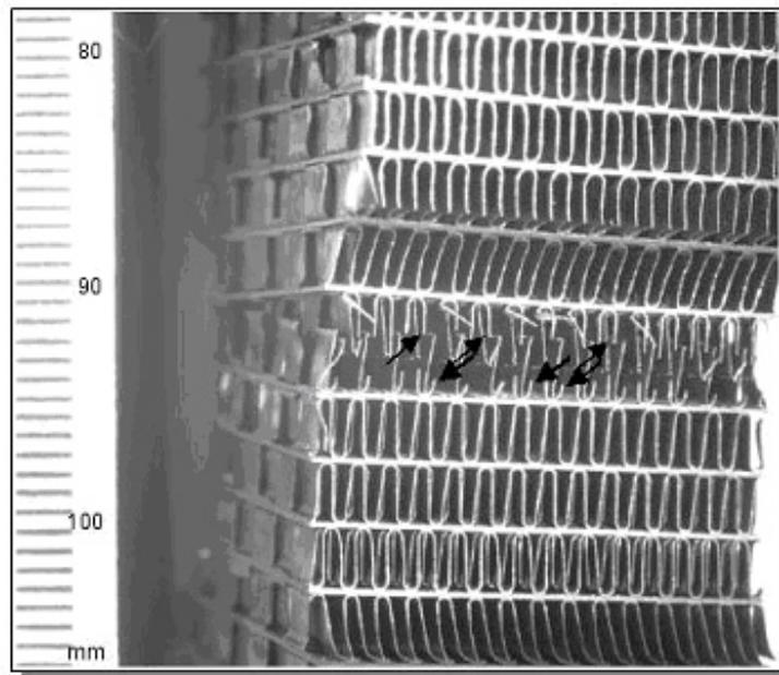
11. Samples of 436 stainless steel plate/fin structure after failure under tensile mechanical testing at 25°C. (a) 25- $\mu\text{m}$  thick MBF-20 foil: Failure occurred in the lean fillets (arrows) formed due to too thin foil used. (b) 50- $\mu\text{m}$  thick MBF-20 foil: Failure occurred in the middle of the fin base metal (arrows) due to large and sufficiently strong joint cross-sections formed using thick brazing foil.<sup>13</sup>
