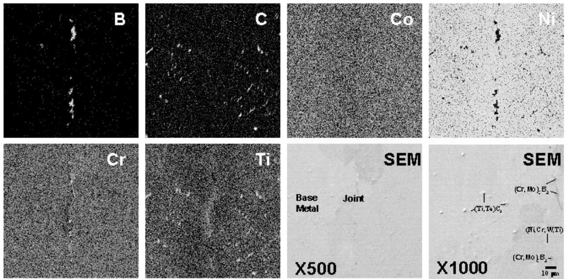
19. Microstructure of and elemental distribution in IN738/MBF-53/IN738 joints brazed at 1170°C for 15 min and annealed at 1070°C for 6 hours.
