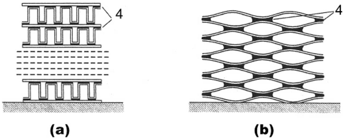
24. Schematics of plate/fin/plate (a) and plate/plate metallic heat exchangers brazed using MBF.
