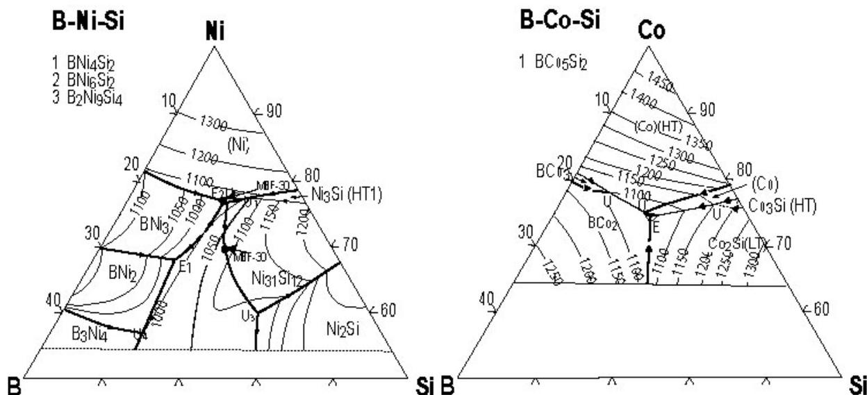
1. Liquidus projections of Ni-B-Si and Co-B-Si phase diagrams<sup>11</sup> and locations of MBF-30 and –35 alloy compositions.
