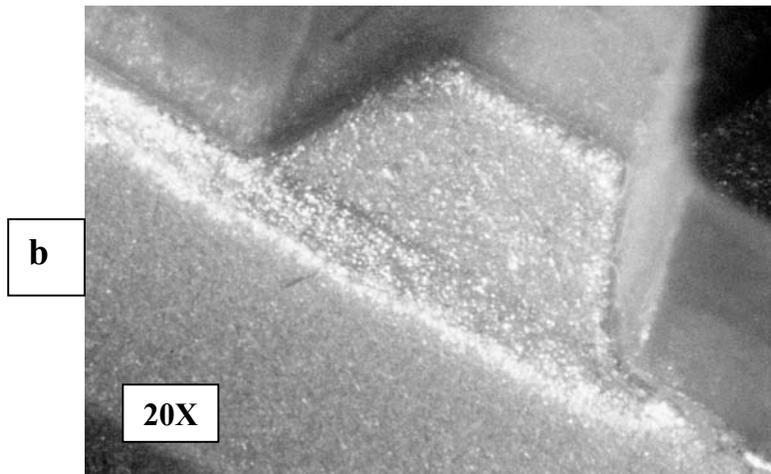
7. IN-738/MBF-100/PM2000 brazed honeycomb turbine seal as viewed for the top (a) and from the side (b). Complete wetting of flat IN-738 surface and formation of very good fillets at PM2000 cell is observed.
