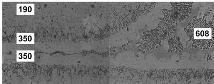
9. Micrograph of a 409/MBF-20/409 joint brazed at 1055°C for 10 min under 50:50 N<sub>2</sub>/H<sub>2</sub> atmosphere having -40°C FP. Numbers indicate Vickers microhardness, kg/mm<sup>2</sup> of some joint area.
