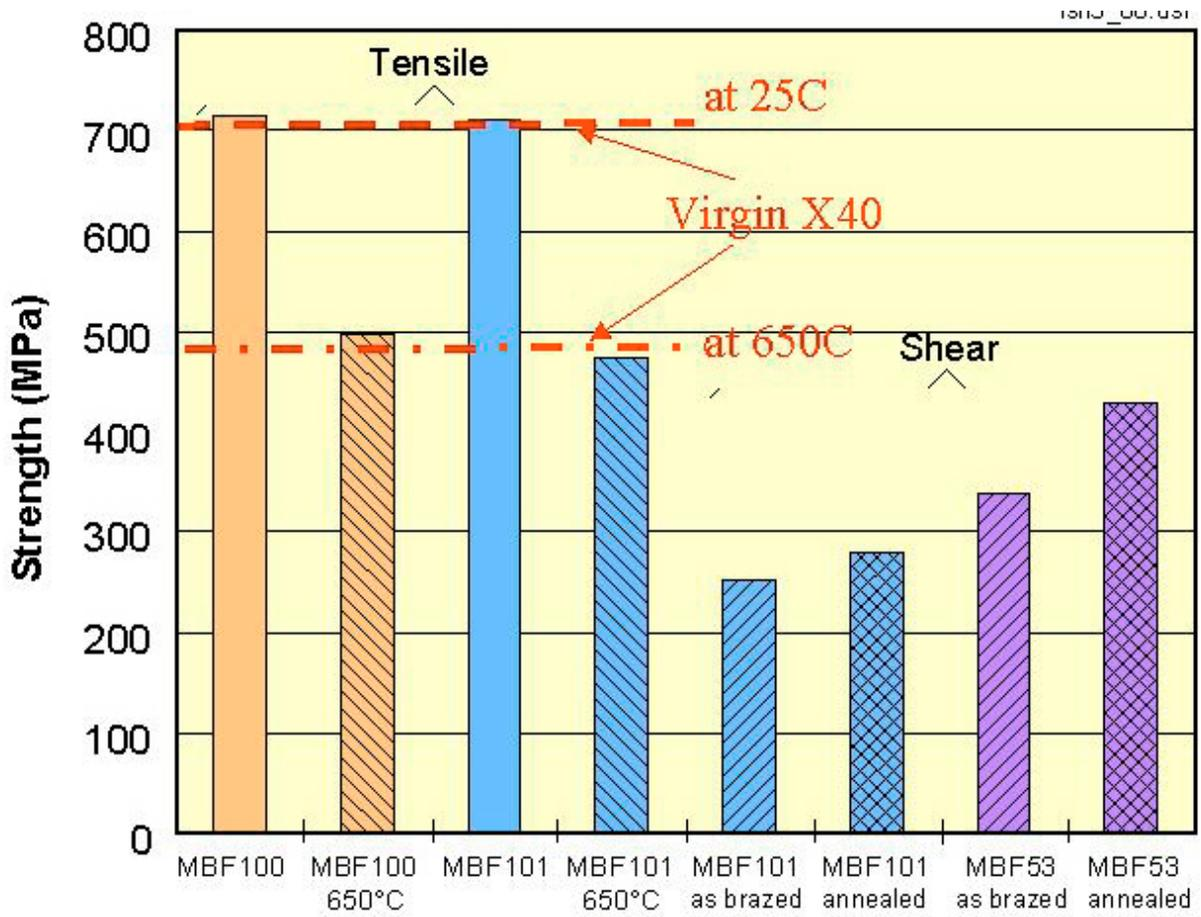
17. Tensile and shear strength of X40/MBF-series alloy joints at 25 and 650°C.<sup>26</sup>
