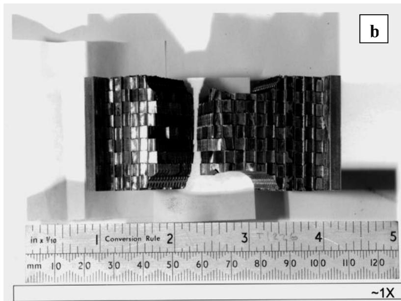
10. Samples of brazed plate/fin 436 stainless steel structures: (a) In the as-brazed state after electroerosion cutting; (b) After failure under mechanical testing in the tensile mode at 650°C.
