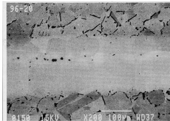
15. SEM micrograph and corresponding x-ray elemental maps of a 316L/MBF-51/316L joint brazed with 2-mil thick foil using a long term brazing cycle. The braze has practically a single-phase (NiCrFeSi) solid solution structure. Boron is diffused into the base metal interface area forming segregated  $Cr_xB_y$  intermetallic crystals at the grain boundaries.<sup>17</sup>
