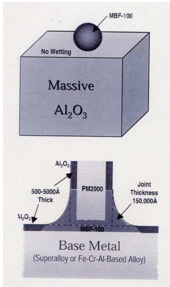
6. Schematics of wetting mechanisms acting during MBF interaction with a massive alumina sample and a base metal part covered by an inherent alumina/titania oxide film.
