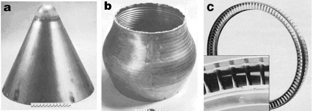
23. Typical aerospace engine parts fabricated using MBF: (a) Exhaust plug for P&W JT9D jet engine<sup>37</sup>; (b) Exhaust plug for GE CF6-80 jet engine<sup>37</sup>; (c) P&W jet engine compressor stator.<sup>36</sup>
