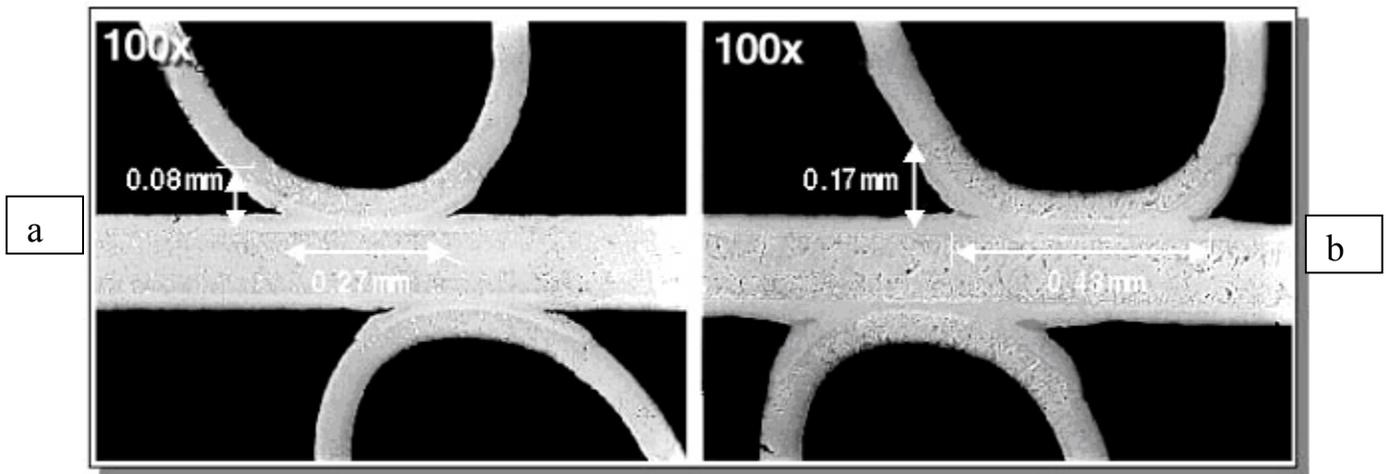
13. Microstructure of two 436 stainless steel plate/fin samples brazed using 25  $\mu\text{m}$  thick (a) and 50- $\mu\text{m}$  thick (b) MBF-20 foil. Note that while inside of the brazes the joint thickness is the same, the cross-section of the 50- $\mu\text{m}$  joint is larger than that of the 25- $\mu\text{m}$  joint. The former is wider and the fillet height is higher. Therefore, the 50- $\mu\text{m}$  joint is substantially stronger.<sup>13</sup>
