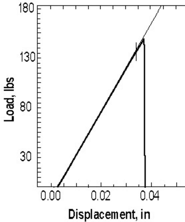
3. Typical load/displacement graph of an MBF-51 specimen in the as-cast state that was mechanically tested with 2.5 mm/min loading rate at 25 °C.
