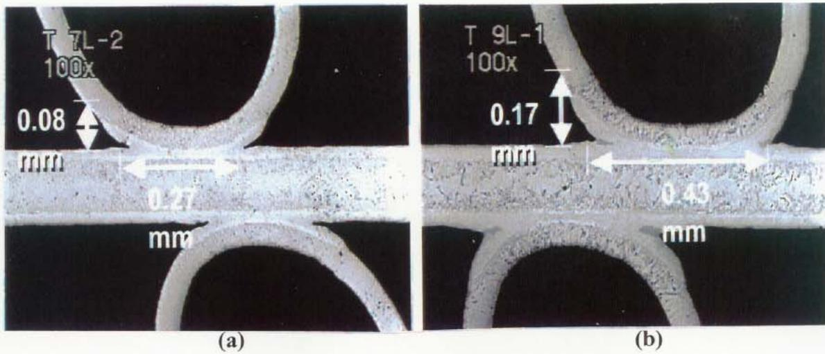
Fig. 2 Microstructure of two 436 stainless steel plate/fin samples brazed using 25  $\mu\text{m}$  (a) and 50  $\mu\text{m}$  (b) thick MBF-20 ribbon. Note that while the joint thickness inside brazes is the same, the joint cross-section is wider and the fillet height is higher when the thicker foil is used.
