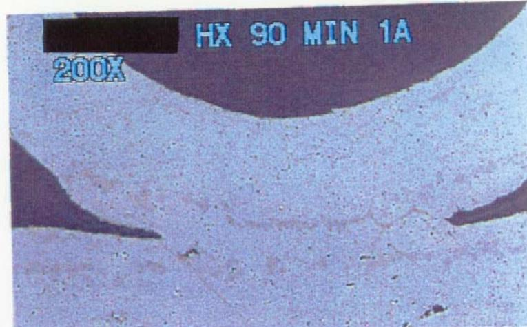
Fig. 6 Micrograph of a Inconel 625 plate/ fin braze of the heat exchanger shown in Fig. 5. The braze has mostly a single phase solid solution microstructure and a favorable morphology of the chromium borides segregated at the joint interfaces.
