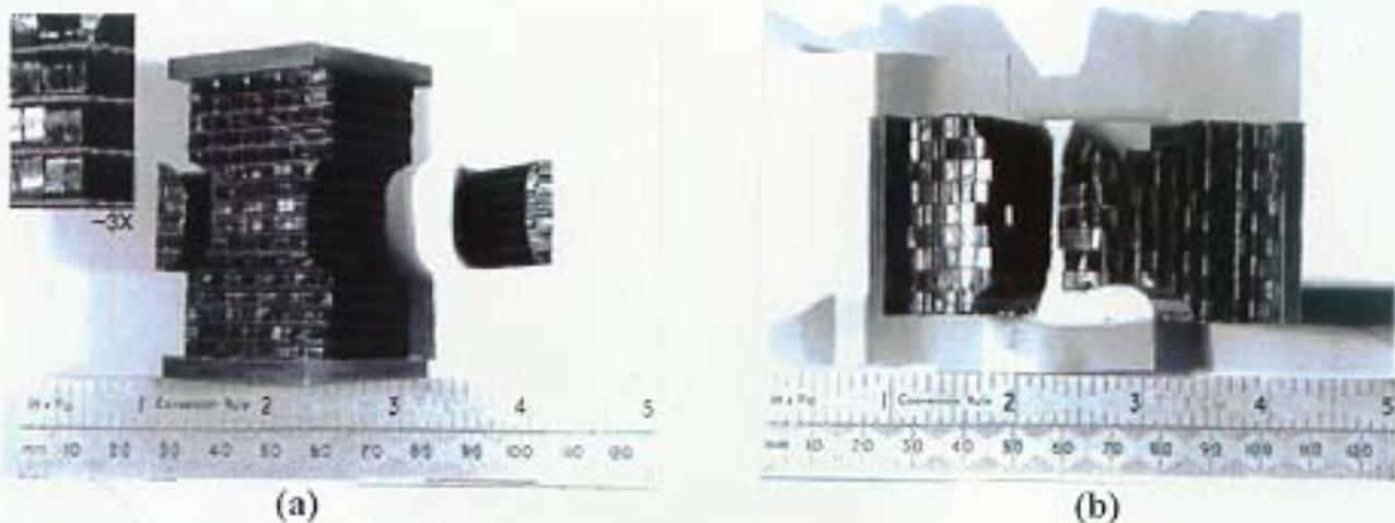
Fig. 1 Samples of a brazed plate/fin structure for mechanical testing after electroerosion cutting (a) and after failure under tensile mode testing at 650°C.
