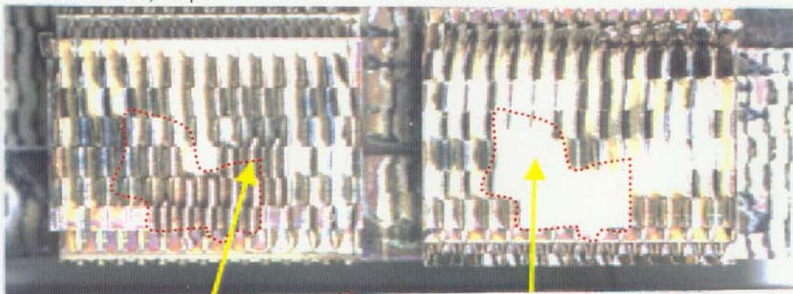
Fig. 4 Two halves of a sample made using 25  $\mu\text{m}$  thick MBF-20 foil. The sample has a large unbraided area due to an insufficient amount of the brazing filler metal.
