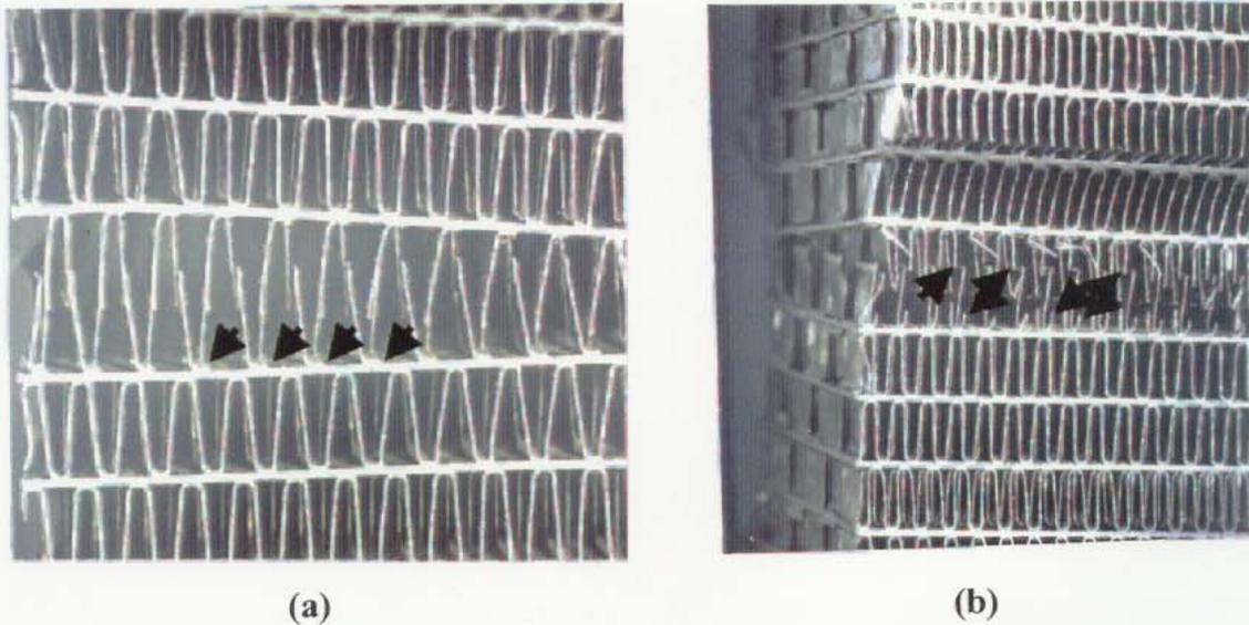
Fig. 3 Failure location in plate/fin structures after tensile mode testing at 650°C. (a) Failure in brazements, 25  $\mu\text{m}$  thick MBF-20 foil was used. (b) Failure in the base metal fins, 50  $\mu\text{m}$  thick MBF-20 foil was used.
